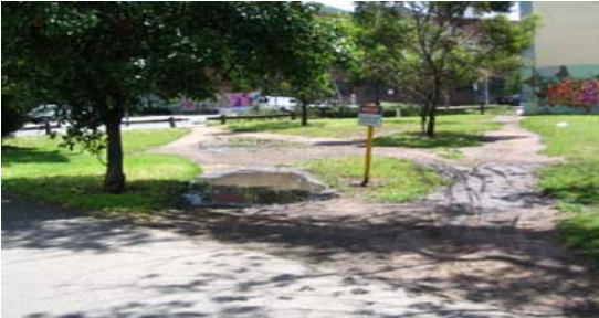
The Infamous Lygon St Swamp, 1. Widen & surface the DIY entrance from lights, 2. Close/narrow the north entrance between footpath & shop 3. Add signage/drainage.
